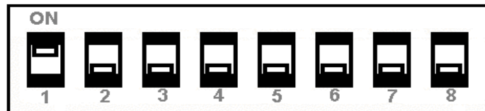
FIGURE 10: DIP SWITCH SETTINGS (SHOWING SETTING FOR IRDA)
